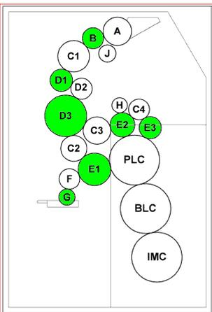
The roller set of the exchange program consist of 7 compounded rollers ( B, D1, D3, E2, E3, E1 en G) according to the picture. The rollers are being delivered in a special crate which is also used for sending the "old" set back.
